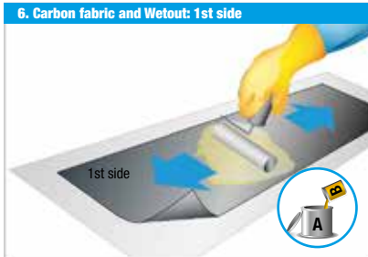
6. Carbon fabric and Wetout: 1st side
