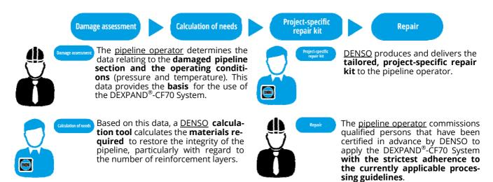
The system has been specifically developed for the repair of pipeline systems. It is not suitable for the repair of leaks. Please refer to the application recommendation available separately.
