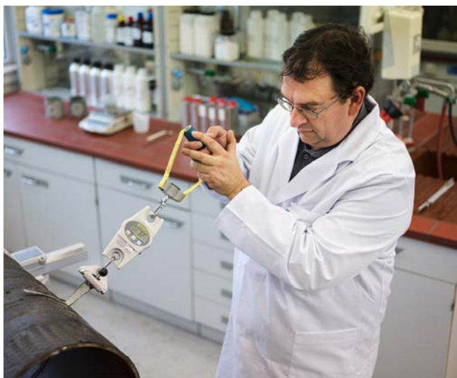
DENSO Group Germany: Peeling test of a 40-year old pipe.
