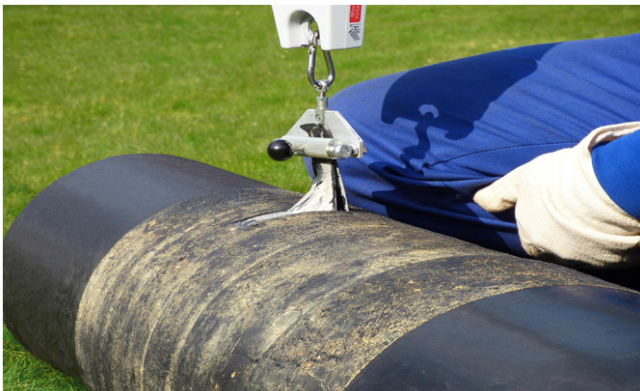
Figure 5. Cohesive separation after 39 years in the field.
